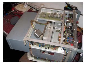
Once removed and the cover slid off the RF unit, it became apparent that the circuit I had did match some of the filter boards. All of the voltages and control lines into the RF unit go through two filter sections. The filters are wound on plastic formers and housed in ferrite pots. I found no less that 12 of these filters to be open circuit.
