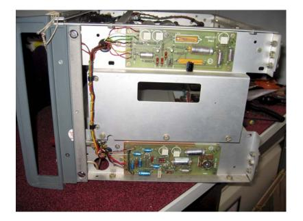
There was still no RF output and no RF indication on the Carrier meter. This left no alternative but to remove the RF unit for examination and repair. The design of the unit makes this a simple task. Removing four screws in the side of the unit allows the whole unit including scale and knobs the be drawn out through the back of the instrument. The module plugs into the carcase via a multi-way plug and socket. Here you can see the RF unit half way out.
