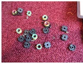
The filters which were removed after being tested with an ohm-meter. Most read High Ks of resistance and should have been in the low 10s of ohms.
